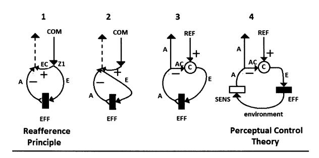
COM = Command; A := afferent signal; E = efferent signal / error signal; EC = efference copy; EFF = effector; AC = afference copy; C = Comparator; REF = Reference signal; SENS = sensor.
